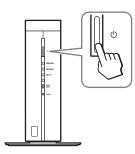
The POWER LED on the front panel of the Base Station lights green. Also, the NET AV LED blinks green until an automatic NetAV check begins.
